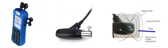
The service life of the OTT MF-Pro should be about ten years. It is an all-electronic device with no moving parts. The sensor is separate from the handset and is also calibrated separately from the handset. This means if the sensor or handset fail, the user could just order the needed component without having to replace the entire setup. This is a relatively new instrument so repair costs are really just estimates at this point.
