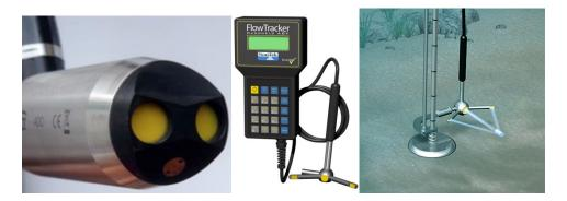
The FlowTracker is based off of Sontek's ADV design with a side looking sensor. It measures a very small space of water four inches away from the center transducer. This offset requires the use of an offset bracket on the wading rod to try to get the sampling volume closer to the position of the rod in the measured vertical. The FlowTracker is kept perpendicular with the tagline and the device measures any angles and corrects for them automatically in the software.
